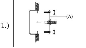
step1:Attach the mounting bracket to the outlet box by using two mounting screws.
