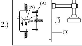
step2:Pull out the source wires from the outlet box. Make wire connections using wire nuts. Attach the fixture grounding wire to the mounting bracket with the green grounding screw, and then connect it to the house grounding wire with a wire nut. Then, attach the body to the mounting bracket, and secure it with one ball nut.
