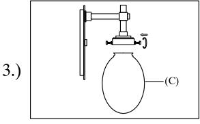
step3:Finally, fix the glass on the body with ball nuts.
